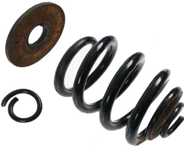
Fig.1: Worn spring seat and broken suspension spring
